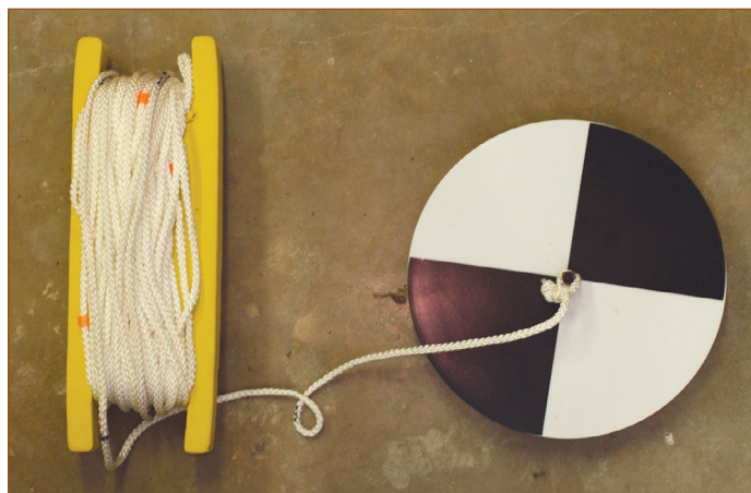
Figure 10. A Secchi disk is useful for measuring water clarity to determine if you need more fertilizer.
